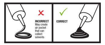
Do not apply mastics in a circle where an air pocket could collect solvents and possibly extract material that could be damaging to the mirror. The best way to apply Premier® Plus from a cartridge is to start from the center and let the mastic naturally expand out as it's being gunned.
